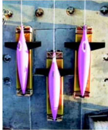
Three Seagliders, seen from above, on the deck of a UW research vessel. Courtesy of J. Osse.
